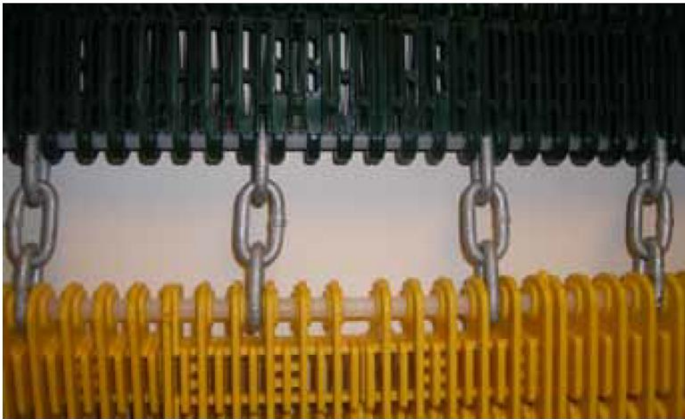
Example of Rigid Chain Pulling Fixture Using Existing Chain
