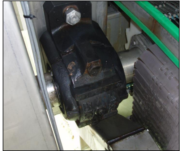
Shafts larger then 3,5" requiring clearance for DTS-C chain
